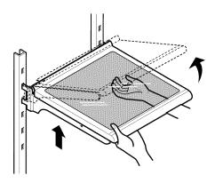
• To reinstall a shelf—Tilt up the front of the shelf and guide the shelf hooks into the slots at a desired height. Then lower the front of the shelf so that the hooks drop into the slots.
